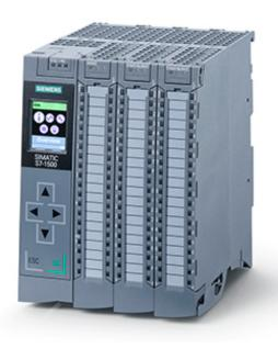
\*\*\* Spare part \*\*\* SIMATIC S7-1500 compact CPU CPU 1512C-1 PN, Central processing unit with work memory 250 KB for program and 1 MB for data, 32 digital inputs, 32 digital outputs, 5 analog inputs, 2 analog outputs, 6 high-speed counters, 4 high-speed counters for PTO/PWM/frequency output 1st interface: PROFINET IRT with 2-port switch, 48 ns bit performance, incl. push-in front connector, SIMATIC Memory Card required
