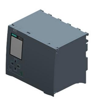
SIMATIC S7-1500F, CPU 1518F-4 PN/DP ODK, Central processing unit with ODK Runtime Interface, work memory 6 MB for program and 20 MB for data, 1st interface: PROFINET IRT with 2-port switch, 2nd interface: PROFINET RT, 3rd interface: Ethernet, 4th interface: PROFIBUS, 1 ns bit-performance, SIMATIC Memory Card required
