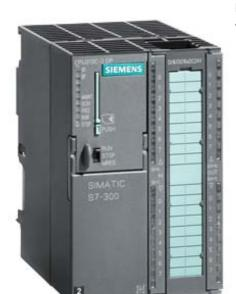
SIMATIC S7-300, CPU 313C-2 DP Compact CPU with MPI, 16 DI/16 DO, 3 high-speed counters (30 kHz), integrated DP interface, Integr. power supply 24 V DC, work memory 128 KB, Front connector (1x 40-pole) and Micro Memory Card required
