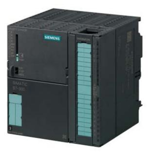
SIMATIC S7-300, CPU 317T-3 PN/DP, Central processing unit for PLC and technology tasks, 1024 KB work memory, 1st interface MPI/DP 12 Mbit/s, 2nd interface DP (drive), 3rd interface Ethernet PROFINET with 2-port switch, Integr. I/O for technology, Front connector (1x 40-pole) and Micro Memory Card min. 8 MB required
